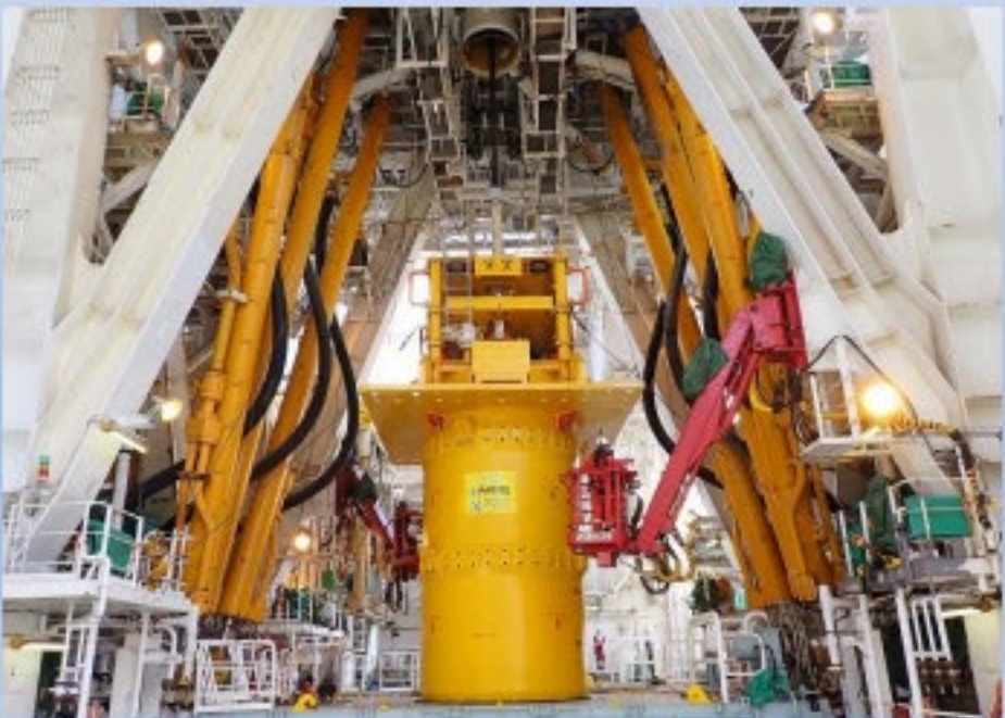
Subsea unit of mineral extraction system on deck of D/V CHIKYU
