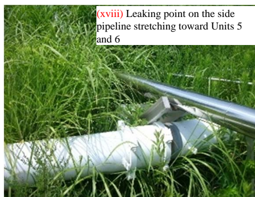
(xviii) Leaking point on the side pipeline stretching toward Units 5 and 6 August 15, 2011 Photographed by Tokyo Electric Power Company
