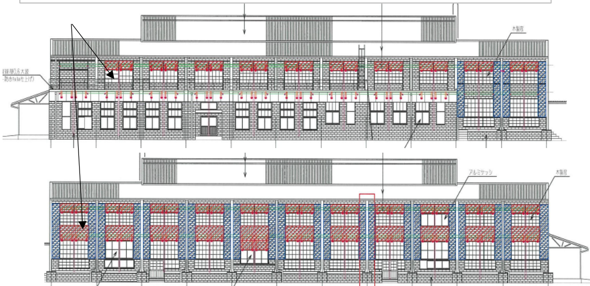
Red parts : All upper slag-brick wall will be reinforced.
