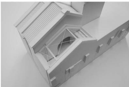
(1) Reinforcement of the roof structure plane of the Storage 1 (former fan room) side bay, looked down from the above
