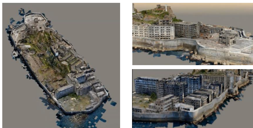
Figure 4: 3-D Model of Hashima Coal Mine made from 3-D laser survey
