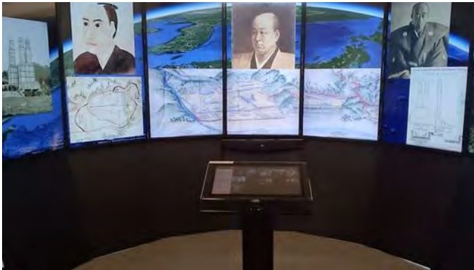
Seven 55-inch displays set vertically controlled by the central touch screen panel.
