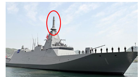
Shipboard composite communication antenna
