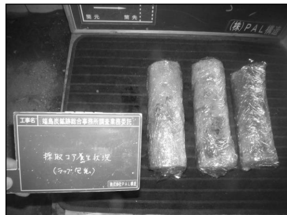
Curing of drilled cores
