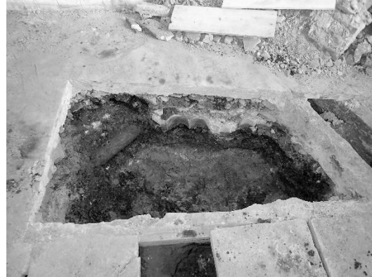
Photo 2-4-92 Exploratory Drilling Site ②, plane view of Layer 2 and soil pipe
