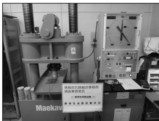
Photo 2-4-70. Performing compressive strength / static elastic modulus tests
